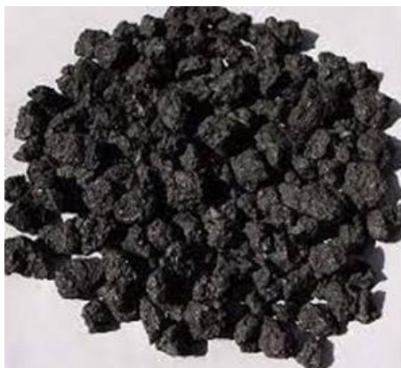
Figure 5. Typical appearance of coarse CPC.
